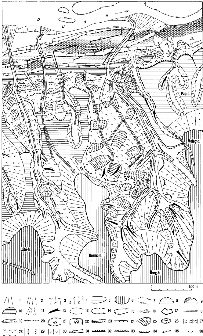
Figure 1. State of slopes: 1 = stable slope; 2 = unstable sliding slope; 3 = active sliding slope; 4 = slope with landslide hazard. Mountain landforms: 5 = interfluvial ridge; 6 = foothill, hillslope. Accumulation landforms: 7 = terrace 1.b; 8 = terrace 2.a; 9 = terrace 2.b; 10 = terrace 3; 11 = debris fan. Channels and valleys: 12 = erosional ravine; 13 = abandoned channels of minor watercourses; 14 = erosional-derasional valley; 15 = derasional valley. Sand forms: 16 = bank dune. Man-made landforms: 17 = settlement; 18 = road; 19 = road cut in loess; 20 = pseudoterrace; 21 = quarry, abandoned; 22 = quarry, upfilled; 23 = canal. Mass movement landforms: 24 = front of slicing landslide; 25 = heap of slicing landslide; 26 = heaps and minor depressions among slips and slumps; 27 = slope affected by slump, in temporary equilibrium; 28 = undulating surface of fossil landslide; 29 = slope wash; 30 = rill erosion; 31 = loess gully; 32 = unstable steep bank; 33 = stable steep bank; 34 = steep bank prone to collapse. Objects damaged by mass movements: 35 = buildings; 36 = embankments, levees
